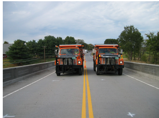
Figure 3: Field testing of Morristown Bridge.
